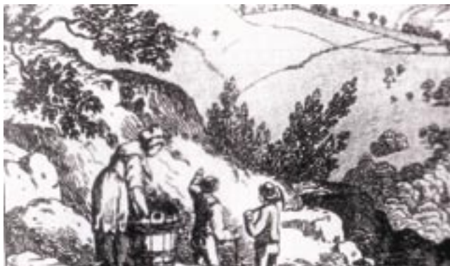
Women did much of the surface work at lead mines. At Gildereye Mine above Matlock Bath in about 1770, a woman sieves ore in a vat of water, while the men gaze into the distance (Lynne Willies collection).
